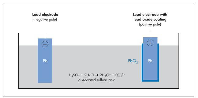
Principle design of a lead-acid battery
