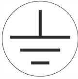
Figure 23: Grounding conductor symbol
