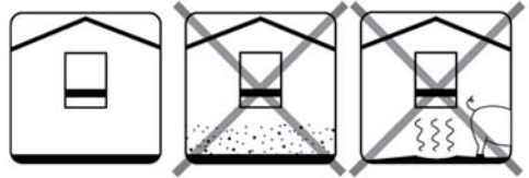
Figure 2.7 Avoid dust and ammonia gases
