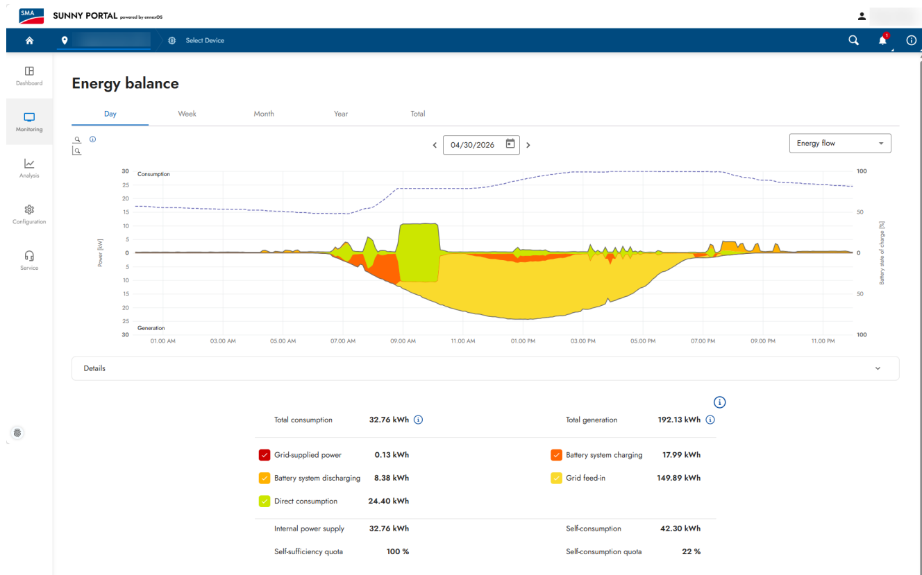
Figure 2: Example of preventing derating losses through targeted battery charging when the export limitation is exceeded (Sunny Portal powered by ennexOS, Monitoring > Energy balance ).
