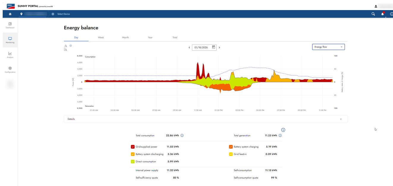
Figure 3: Visualization of peak load shaving in Sunny Portal powered by ennexOS ( Monitoring > Energy balance ).
