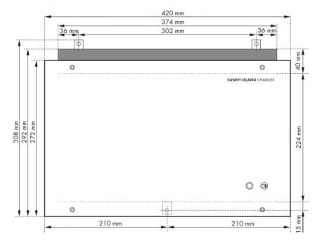
Drill the holes (diameter: at least 8 mm) at the indicated positions and use wall anchors (at least M8).
