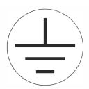
Figure 25: Grounding conductor symbol
