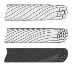
Figure 31: Cables with different conductors (from top to bottom): multi-strand, fine-strand and extra fine-strand
