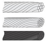
Figure 24: Cables with different conductors (from top to bottom): multi-strand, fine-strand and extra fine-strand
