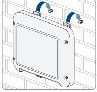
6. Tighten the screws hand-tight using a ratchet or box wrench. When doing this you can compensate for any misalignment of the drill holes by aligning the metal brackets accordingly.
