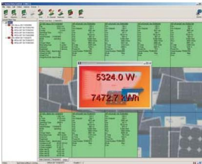
If required, the PC can also be connected with the Sunny Boy Control via modem. By connecting several Sunny Boy Controls, it is possible to monitor large scale plants with more than 50 Sunny Boys or Sunny Mini Centrals.
