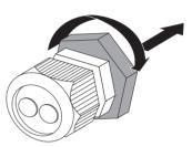
5. Place the cable gland into the enclosure opening of the inverter and fastening it along with the counter nut from inside.
