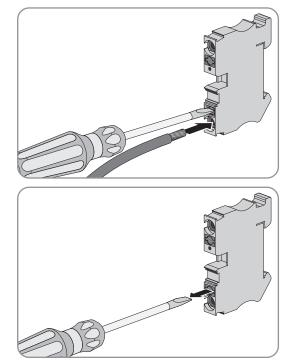
3. Pull the screwdriver out of the clamping contact.
