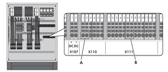
Figure 8: Overview of the provided jumper wires when installing the Multicluster-Box without Grid-Connect-Box
