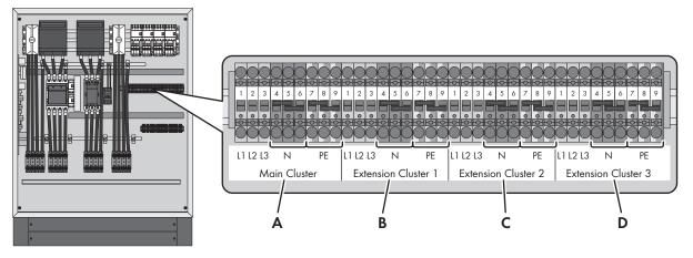
Figure 9: Overview of the spring-cage terminals for connecting the power cables of the Sunny Island inverters
