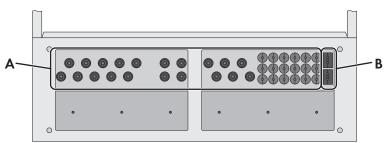
Figure 7: Enclosure openings in the bottom of the Multicluster-Box
