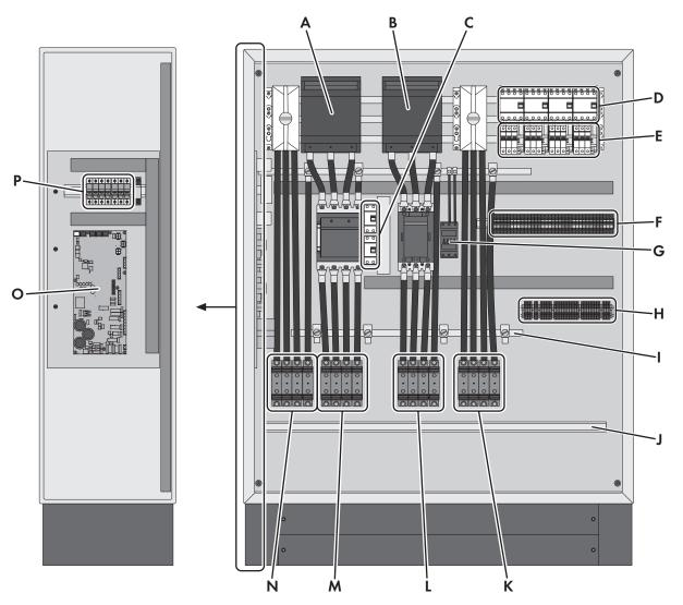
Figure 6: Components and terminals inside the Multicluster-Box
