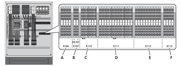
Figure 10: Overview of spring-cage terminals for connecting the control cables
