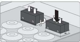
4. Loosen the screws of the two-part cable feed-through and remove the half without the T-shaped fastening pieces.
