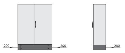
Figure 5: Recommended clearances(Dimensions in mm)
