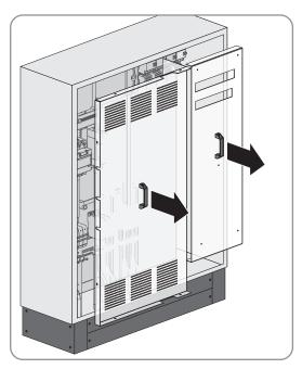
3. Retain the protective cover and the fastening screws for later use. In this way, the protective cover can be mounted at a later time and thus the Multicluster-Box recommissioned.
