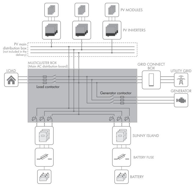
Figure 3: Circuitry principle of a multicluster system - example with Multicluster-Box
