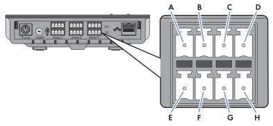
Figure 17: Pin assignment of the pin connectors on the bottom enclosure side
