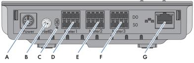
Figure 14: Terminals on the bottom of the enclosure
