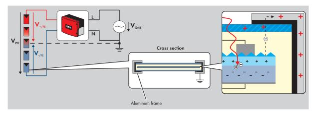
Figure 1: Build-up of electrical charges due to a leakage current between the PV cell and module frame
