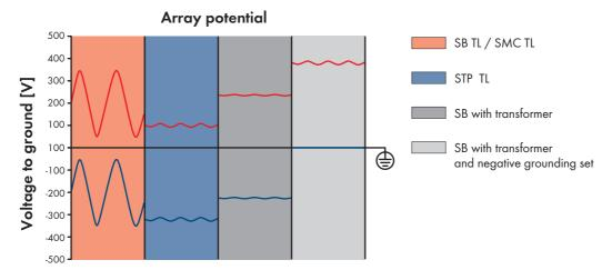
Figure 3: The potential of the lowest (blue) or highest (red) PV module in a string (see also figure 1) depends on the inverter used and whether an array pole is grounded. Example for MPP voltage of 400 V.
