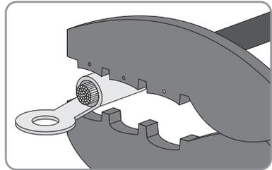
3. Connect the grounding conductor to the grounding terminal. Observe the position of the terminal (see Section 6.1, page 26). Observe the order given below and hand-tighten the fastening screw (torque: 0.8 Nm):
