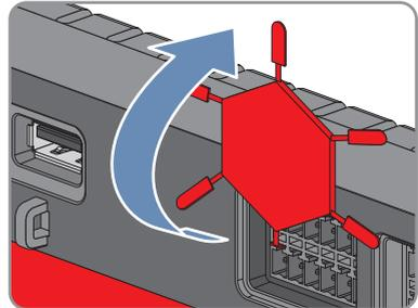
3. On the multipole plug, remove the key from the conductor entry that will receive the coded pin when connected to the Cluster Controller.
