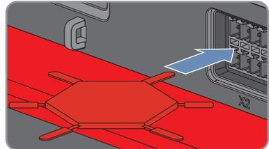
2. Remove the coding tab from the coding element by snapping it off.
