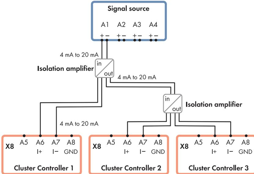
Figure 25: Transmission of analog current signals for active power limitation to three Cluster Controllers via isolation amplifiers (example)
