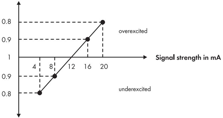
Figure 30: Interpretation of the signal strength as displacement power factor  $\cos \varphi$ **Procedure:**
