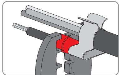
3. Trim unneeded insulated conductors flush with the cable sheath.
