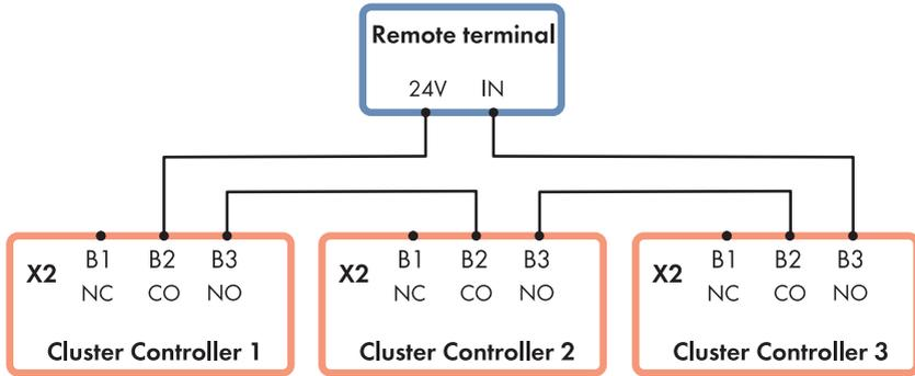
NC = Normally Closed (back contact), CO = Change Over (change-over contact), NO = Normally Open (front contact)
