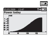
If you are charging the batteries via the Sunny Beam USB connection, the Sunny Beam will visualize the charging process by displaying the battery symbols one after the other.
