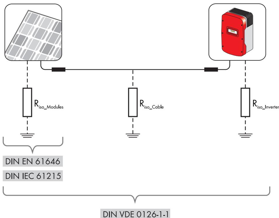
In transformer-less inverters, the continuous measurement of  $R_{iso}$  in operation is not possible due to this missing galvanic isolation. Thus transformer-less inverters must measure the  $R_{iso}$  before grid connection and monitor the residual current during operation.
