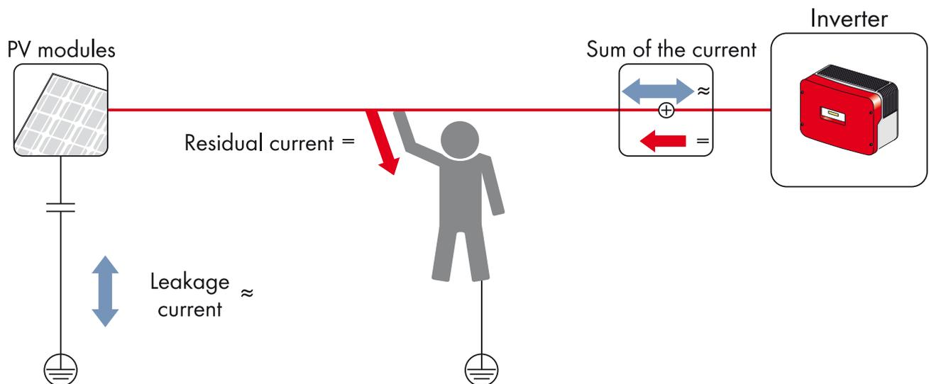
Figure 3: Formation of residual current through contact between a grounded person and a live line
