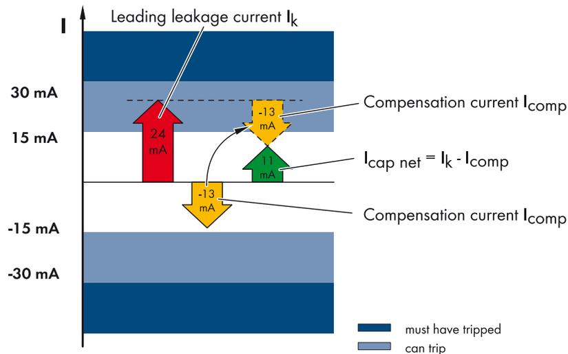
Figure 5: Diagram of tripping behavior with compensation current
