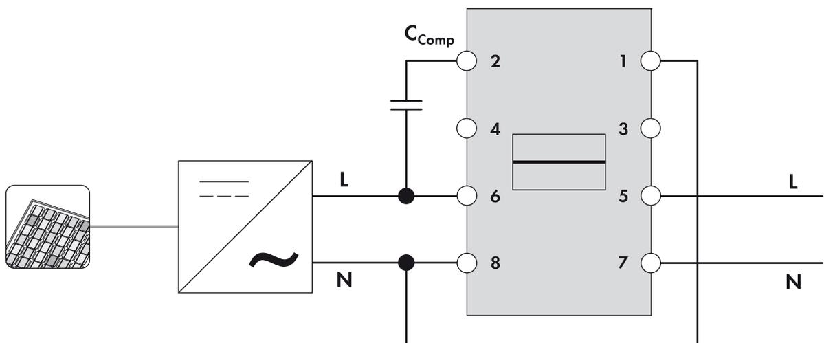
Figure 6: Schematic illustration of the connection of a compensation capacitor to the residual-current device
