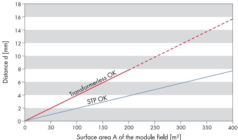
Figure 7: Minimum distance of PV cells to grounded surfaces for single-phase and three-phase transformerless inverters. The operating point of a PV system should always be above the corresponding limit line.
