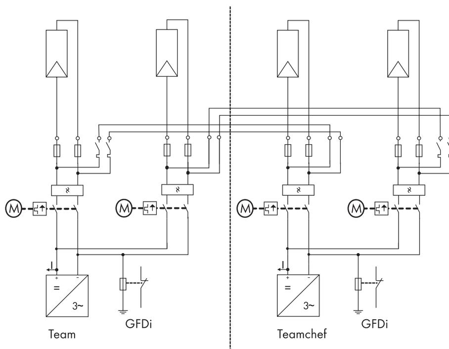
Figure 4: Position of the GFDI in the Sunny Central 500 / 560HE
