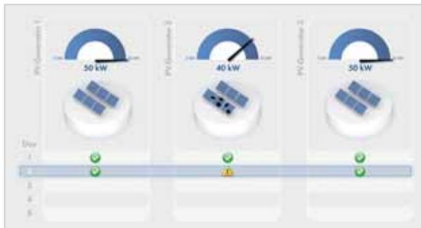
Optiprotect can detect temporary shading based on previous plant data. This makes it possible to distinguish between temporary disturbances and actual errors. False alarms are avoided.
