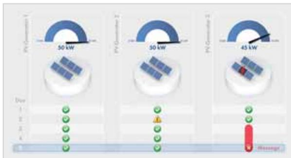
Optiprotect can reliably detect and report string failures. Only when a failure is reported will a service call be necessary.
