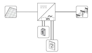
Figure 1: Principle of a PV system for secure power supply
