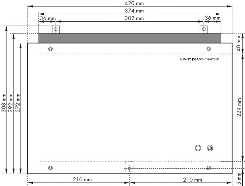
2. Drill the holes (diameter: at least 8 mm) at the indicated positions and use wall anchors (at least M8).
