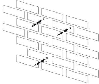
3. Screw the charge controller onto the wall using the three mounting plates. Use fastening material suitable for the surface.
